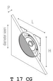
da incasso su cartongesso in-wall, for wall made of plaster/paperboard
